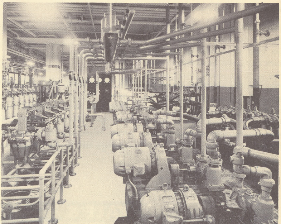
Type 80-BVM and 100-CVM units blending basic oil stocks with additives at the new installation.
